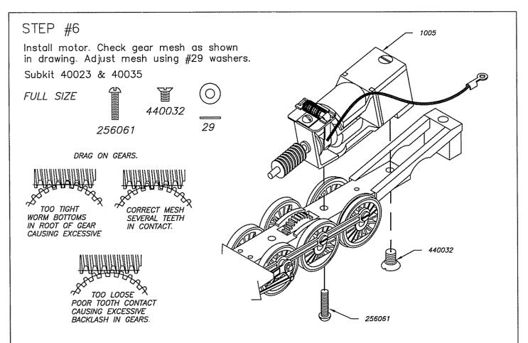
Too Tight — put a #29 washer between front motor bracket and frame
