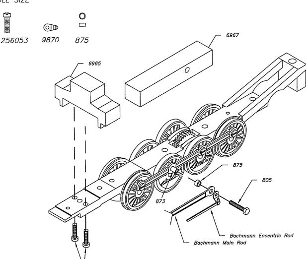
Glue Bachmann cylinder cover and valve gear assembly to the cylinder spacer #6965 (Goo or Ambroid original cement recommended)
