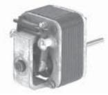
**DC-84 MOTOR** .009 HP at 9,500 RPM. Dimensions: 1 11/16" long x 1 11/16" wide x 1 3/8" high; 1/8" shaft extending approximately 1/2" on both ends. Wound for 12 volt DC operation.
